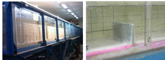
Fig. 2. Photos of laboratory setup, a) Settling tank (left), b) Baffle (right).
