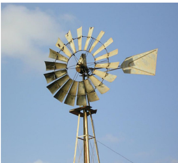
Fig. 1 Typical American-type wind-driven water pump
