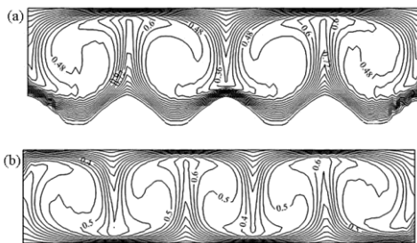
Figure 6. Isotherms comparisons of collectors, in the cases of Ra = 10^5 , As = 2 and Ar = 0.15 , between: (a) Wavy absorber collector, and (b) Flat absorber collector.
