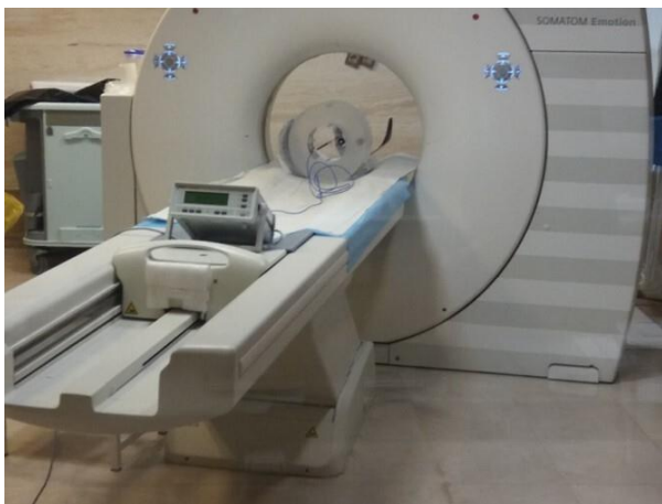
Figure 4. CTDI phantom in position with the pencil ionization chamber connected to the electrometer and positioned in the center hole of the phantom for CTDI_{100,c} measurement
