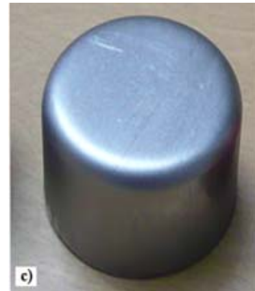
Fig. 5 Photograph of the hydroformed work pieces obtained from experiments (a) parabolic cup, (b) hemispherical cup, (c) cylindrical cup
