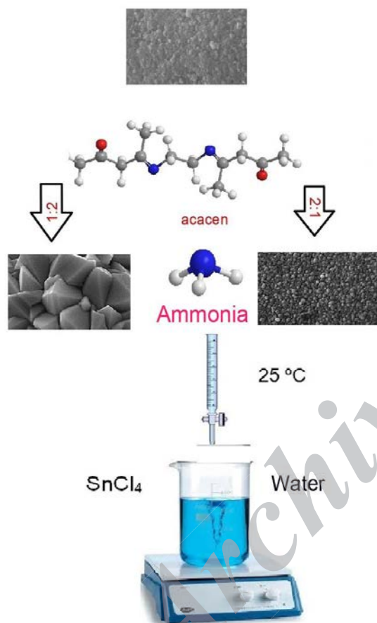
Fig. 1. Schematic diagram of preparation of SnO 2 nanoparticles
