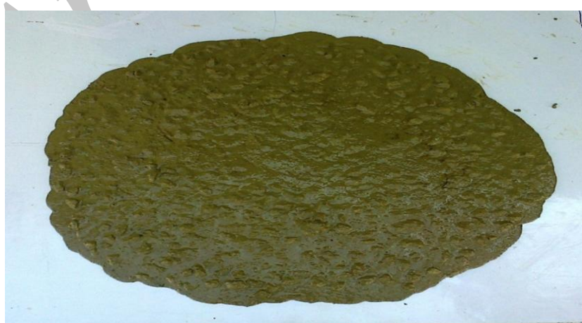
Figure 3. Slump flow test
