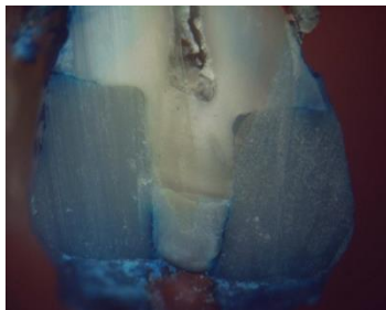
Figure 5 - Dye penetration in samples 3 and 4 in group 4
