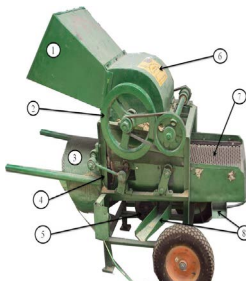
Figure 1. The chickpea thresher: (1) Funnel feed; (2) Flywheel; (3) Blower; (4) Main frame; (5) Electrical motor; (6) Threshing drum; (7) Screen, (8) Outlet for clean seeds.
