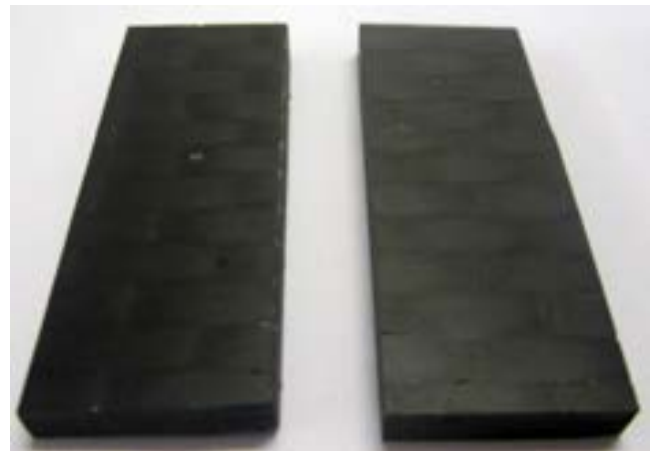
Fig. 5. Prepared composite specimens.
