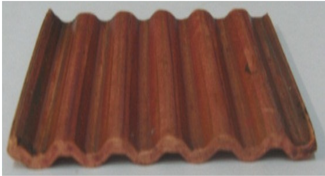
Fig. 5. Copper sample after pressing the 5 times.
