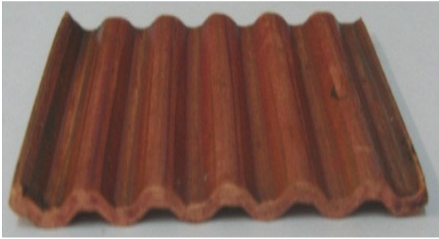
Fig. 5. Copper sample after pressing the 5 times.
