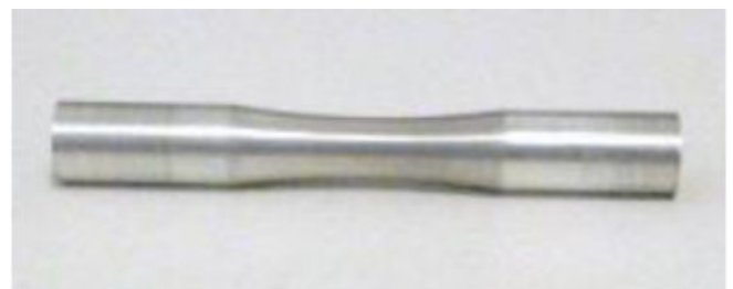
Fig. 5. Round specimens used for extracting S-N curve of AZ31B [10].
