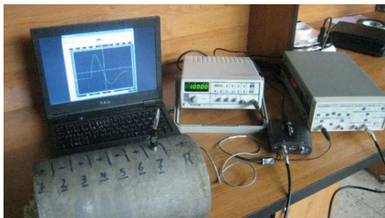
Fig. 7 System and pulse eddy current test equipment
