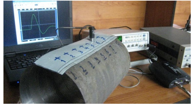
Fig. 12 Corrosion tests on three layers insulation on a gas pipe
