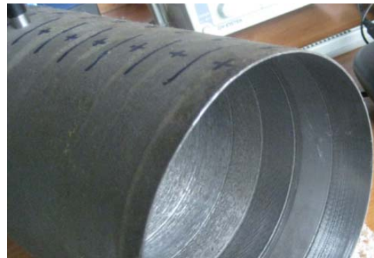
Fig. 8 Simulated corrosion with different thickness on gas pipe
