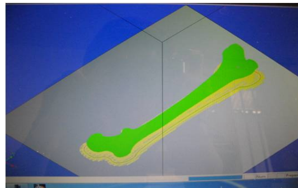
Fig. 13 Layered model in the RP system's software [27]
