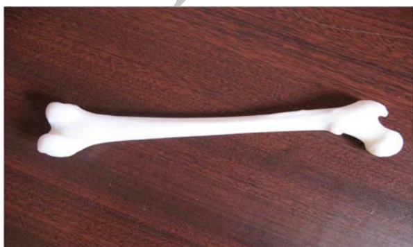
Fig. 17 Completed part with finished surfaces [27]
