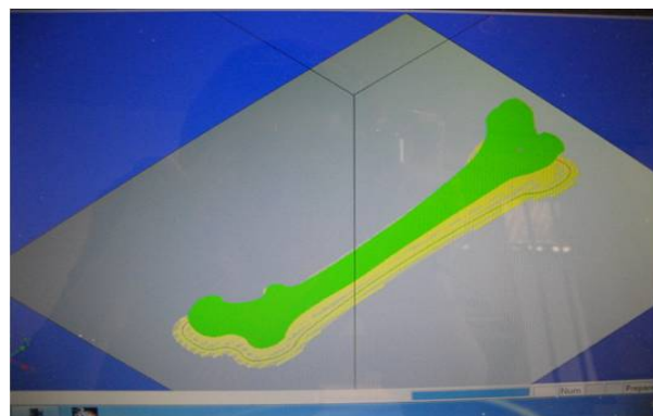
Fig. 13 Layered model in the RP system's software [27]
