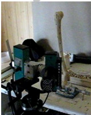
Fig. 6 Optical measurement of femur bone [27]
