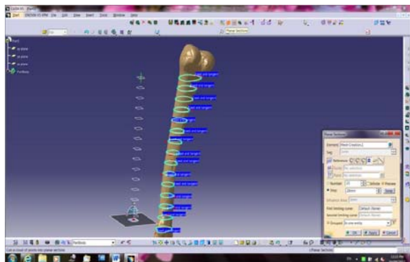
Fig. 11 Contour generation of meta and diaphysis [27]
