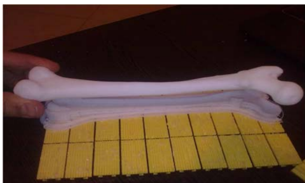
Fig. 16 Part's separation from its support [27]
