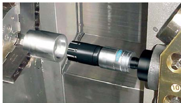
Fig. 2 Entering the roller burnishing tool into the work piece (Performance of ECOROLL Company)
