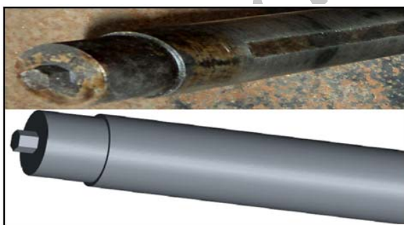
Fig. 3 Geometry of the hexagonal tool pin profile used in the present study
