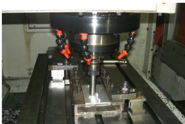
Fig. 5 FSW Processing set-up
