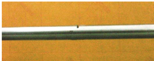
Fig. 9 Transverse crack like fault made on the shaft
