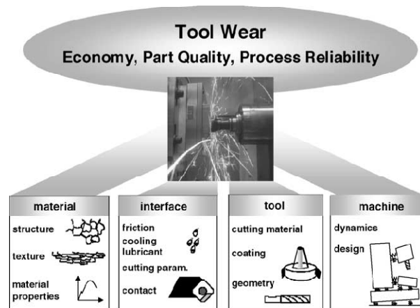
Fig. 2 Four functional elements influencing tool wear in machining processes
