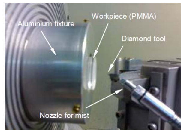
Fig. 2 Close set up view of Diamond Turning Operation
