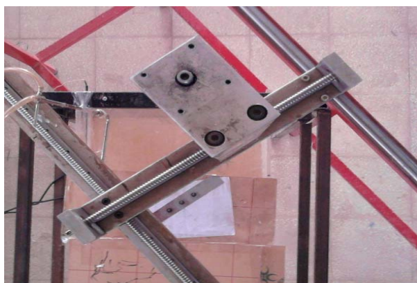
Fig. 2 location of probe displacing system on compressor cascade
