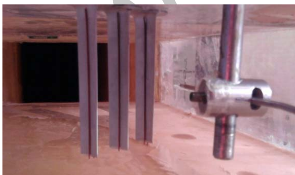
Fig. 3 Placing tripping wires on compressor's blades in wind tunnel
