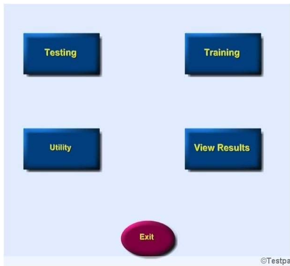
Fig. 5 Start form. This form is executed at the software startup and takes the stabilometer to a fixed situation. Then choosing one of Testing or Training buttons launches the proper mode. It is also possible to view the previous results of a specific patient or perform the settings of CDP.
