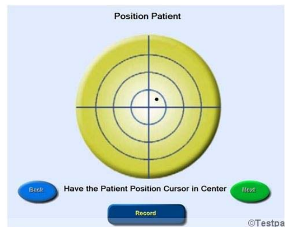
Fig. 6 The Centering Process form. The person is engaged to position feet such that the black point of COP on the circle target intersects the origin. Then pressing Record stops the process and coordinates of the feet are imported by the operator. This process is called Centering
