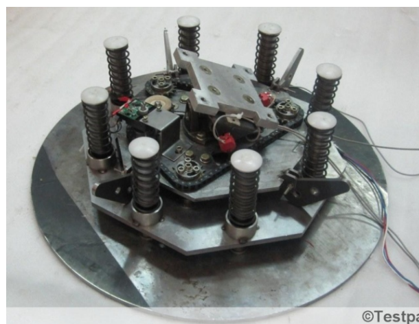
Fig.1 The stabilometer used in the study without outer frame and upper plates
