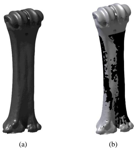
Fig. 12 (a) Point clouds of COMET5 TM scanner, (b) consistency of point clouds with output of the developed program as a color coded image
