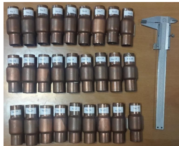
Fig. 4 Formed specimens using the rotary tool
