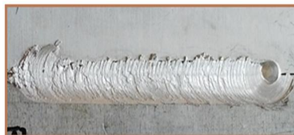
Fig. 2 Lateral flash in the joint FSW
