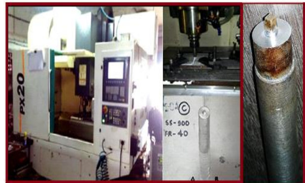
Fig. 1 Friction stir welding on VMC machine with FSW joint
