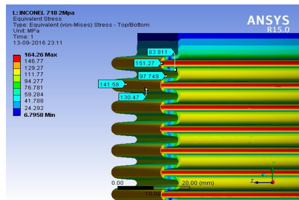
Fig. 19 Stress distribution at Pressure 20 Bar
