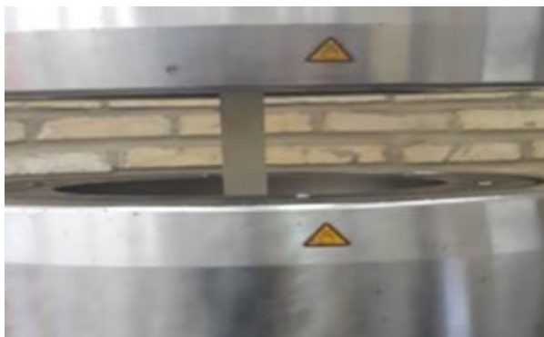
Fig. 2 Tensile test on a sample by INSTRON device.
