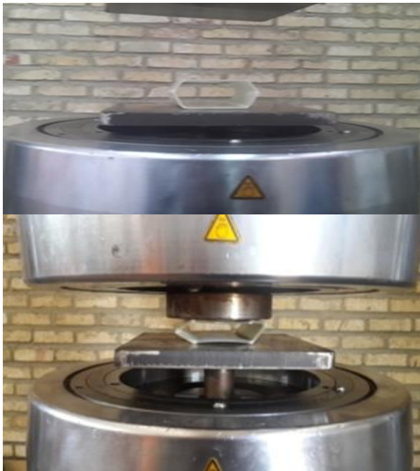
Fig. 5 Rectangular composite tube before and after lateral loading.
