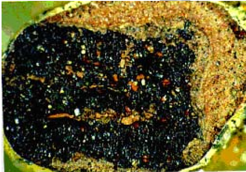
Fig. 28. An ellipsoidal multi stage rim, complex and secondary pisoid lag formed over a widely varying time periods (field of view is 3.5 mm)
