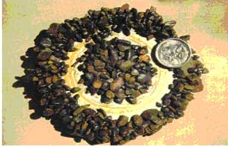
Fig. 25. Pisoid type magnetic (maghemitized) lag with highly polished and varnished surface, from surface above the sample site in picture 21 (attracted by a hand magnet)
