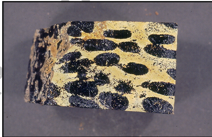
Fig. 2. Elongated chromite nodules hosted in serpentinized dunites of the Forumad ophiolite. These nodules have been stretched, showing spindle-like form.
