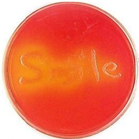
Fig. 1. The phenol red plate assay to show extracellular lipase production of the strain NEB-1. The colonies with obvious color change from pink to yellow reveal production of free fatty acid in the olive oil plate after hydrolysis.
