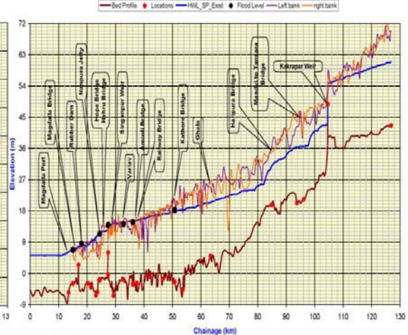
Fig. 10. Water Profiles of Tapi River for Discharge 8 Lakh Cusecs during Spring Tide at HWL
