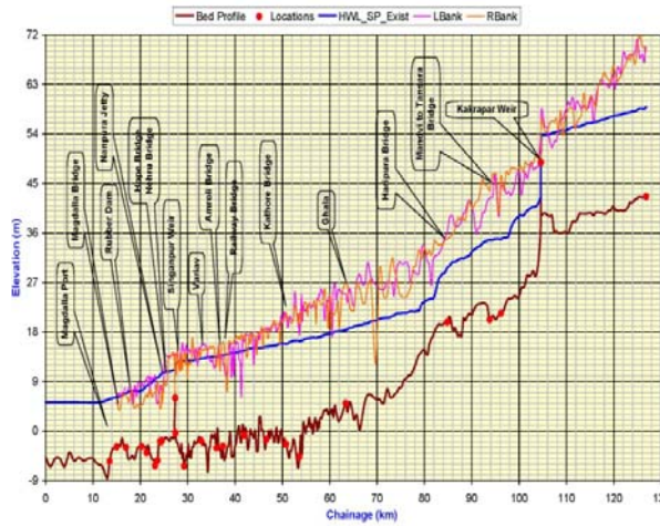
Fig. 7. Water Surface Profiles of Tapi River for Discharge 3 Lakh Cusecs during Spring Tide at HWL
