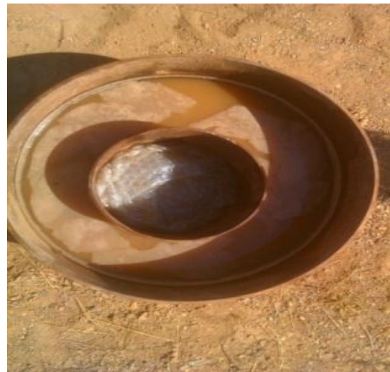
Fig. 3. Double rings for soil infiltration measuring
