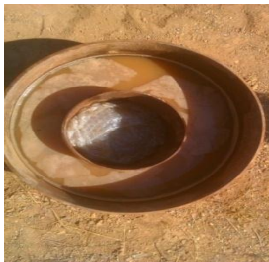
Fig. 3. Double rings for soil infiltration measuring
