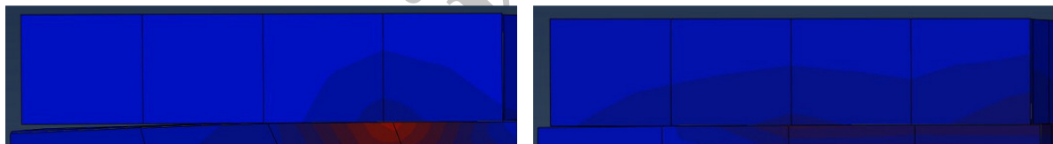
Fig9. contact situation between disk and pad after 1.6 sec in steel and FGM disks
