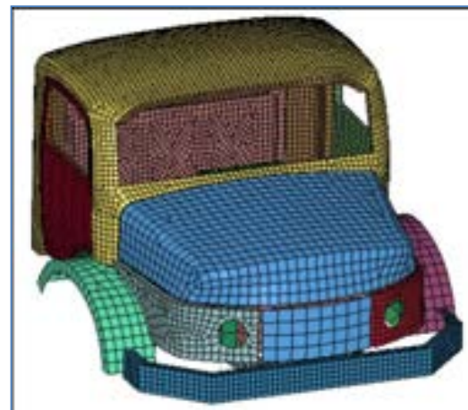
Fig6. Final finite element model of the truck
