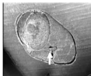
Figure2: Type 3 failure mode (Mix). The arrow shows the cohesive failure in Panavia F.2 cement.
