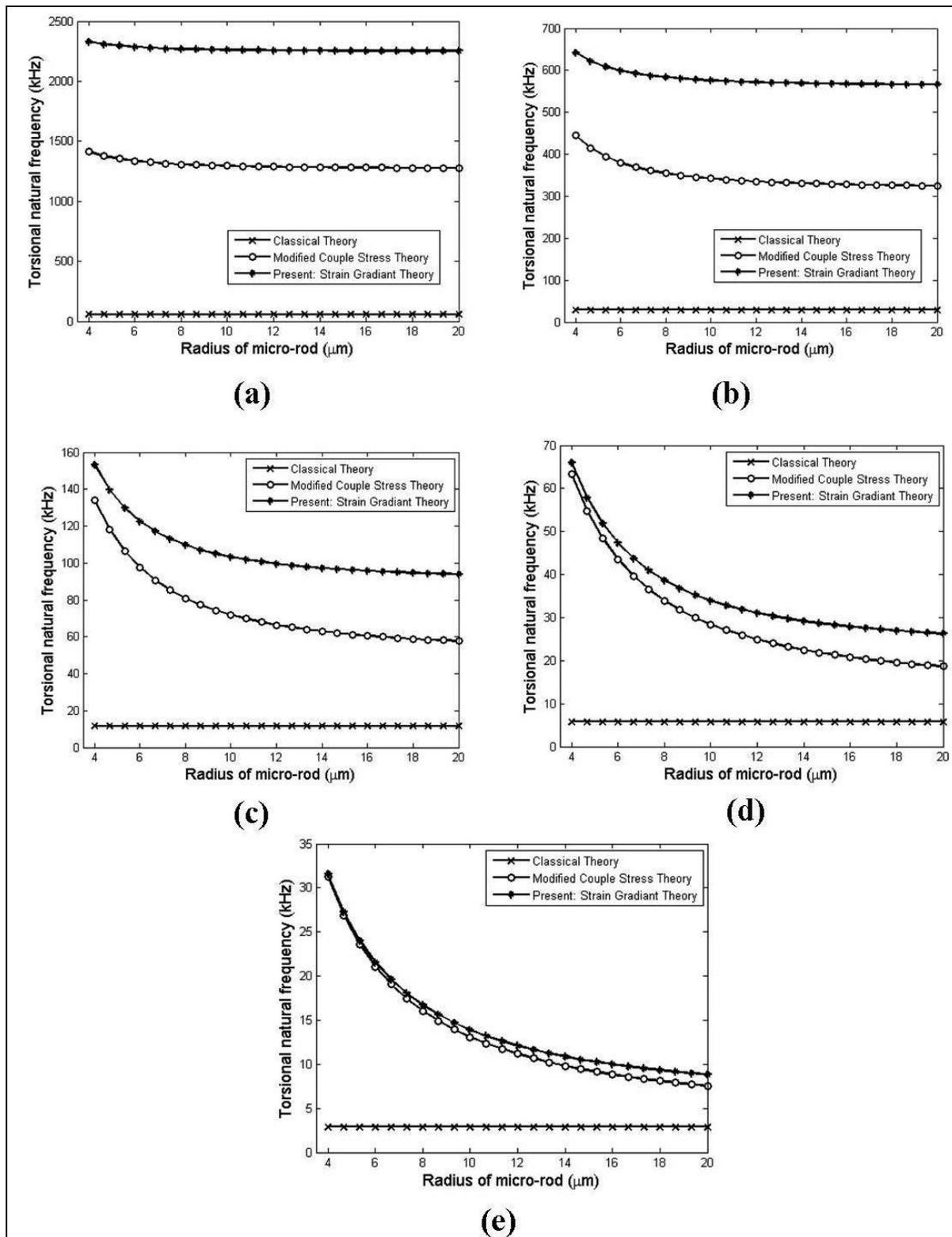
Fig. 5. Variation of fourth torsional natural frequencies of micro rod with radius for various lengths (a)  $L = 5 \mu\text{m}$ , (b)  $L = 10 \mu\text{m}$ , (c)  $L = 25 \mu\text{m}$ , (d)  $L = 50 \mu\text{m}$ , (e)  $L = 100 \mu\text{m}$ .
