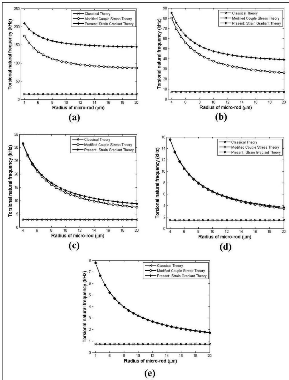
Fig. 2. Variation of first torsional natural frequencies of micro rod with radius for various lengths (a)  $L = 5 \mu\text{m}$ , (b)  $L = 10 \mu\text{m}$ , (c)  $L = 25 \mu\text{m}$ , (d)  $L = 50 \mu\text{m}$ , (e)  $L = 100 \mu\text{m}$ .
