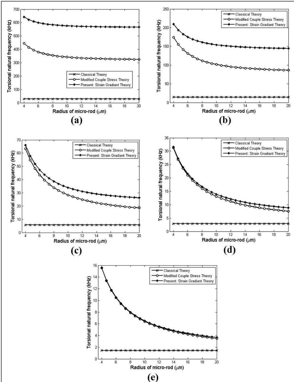
Fig. 3. Variation of second torsional natural frequencies of micro rod with radius for various lengths (a)  $L = 5 \mu\text{m}$ , (b)  $L = 10 \mu\text{m}$ , (c)  $L = 25 \mu\text{m}$ , (d)  $L = 50 \mu\text{m}$ , (e)  $L = 100 \mu\text{m}$ .
