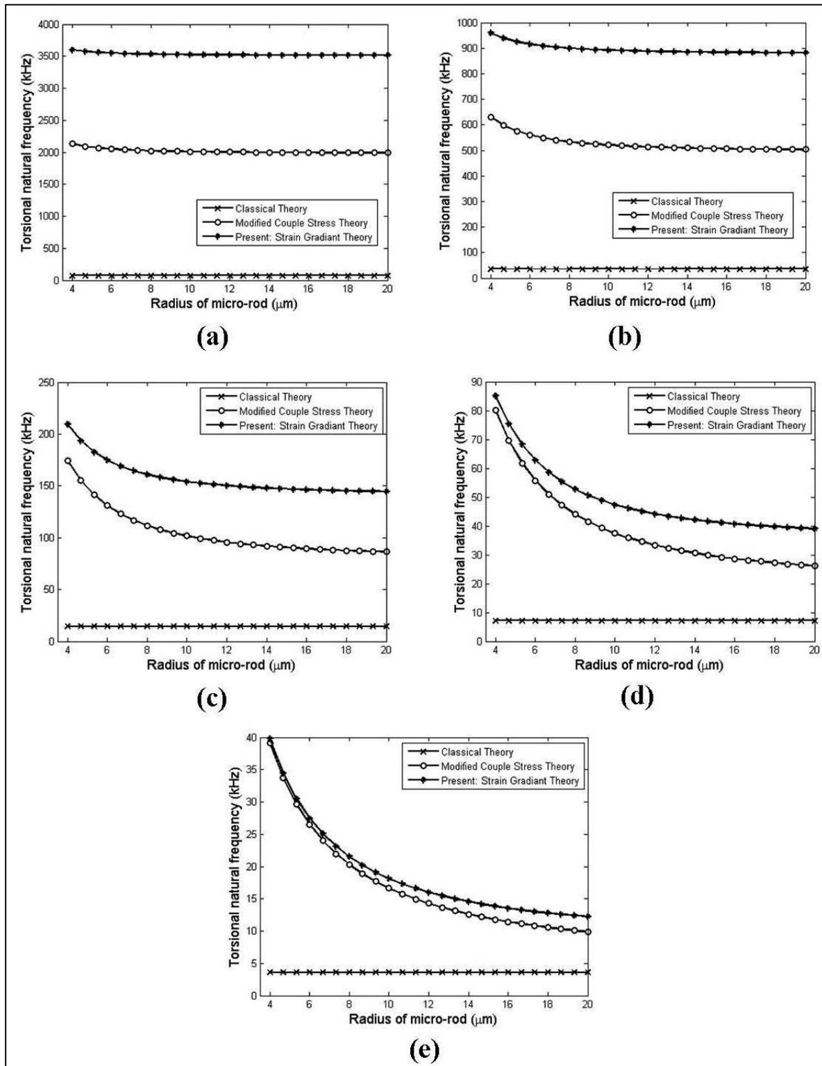
**Fig. 6.** Variation of fifth torsional natural frequencies of micro rod with radius for various lengths (a)  $L = 5 \mu\text{m}$ , (b)  $L = 10 \mu\text{m}$ , (c)  $L = 25 \mu\text{m}$ , (d)  $L = 50 \mu\text{m}$ , (e)  $L = 100 \mu\text{m}$ .
