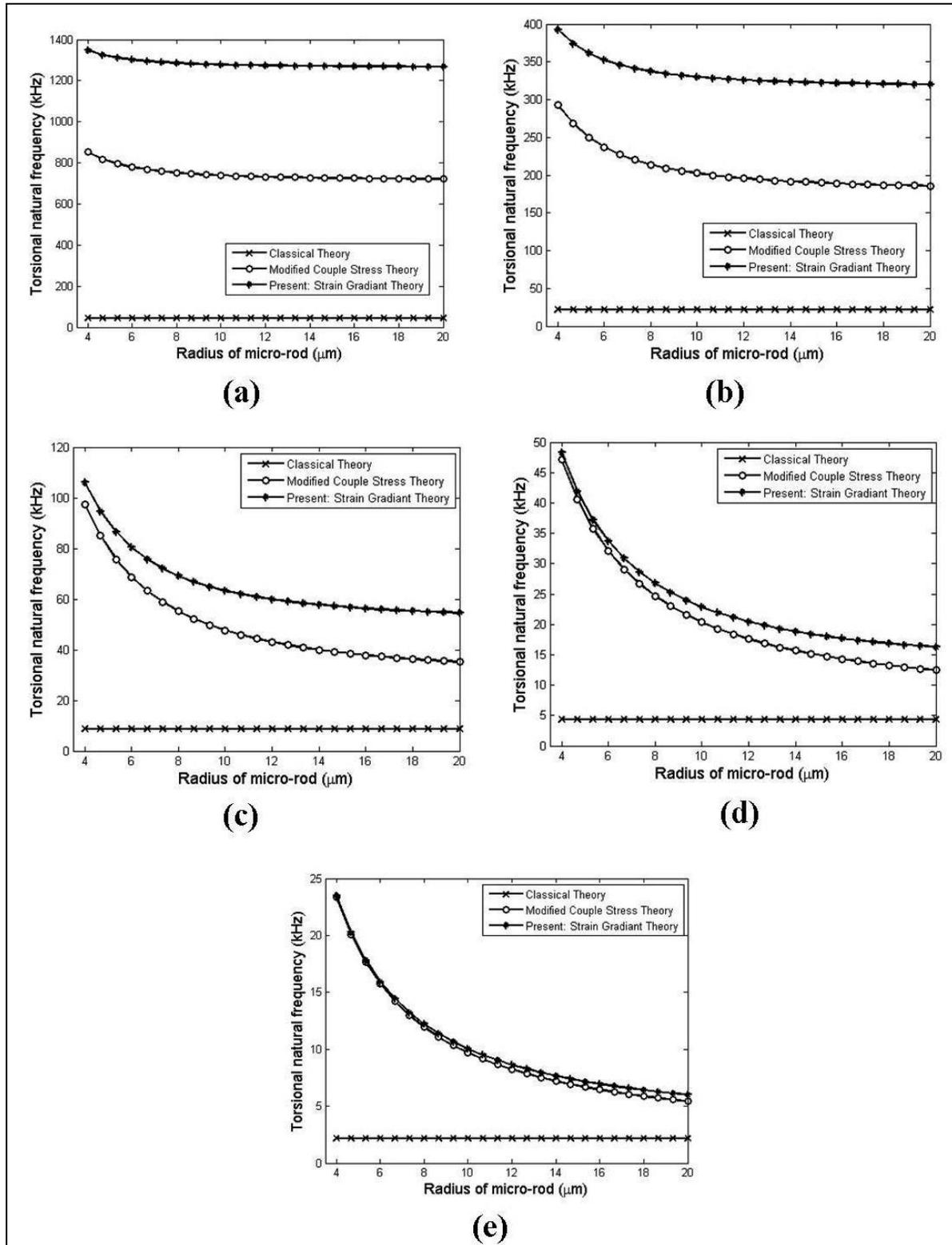
Fig. 4. Variation of third torsional natural frequencies of micro rod with radius for various lengths (a)  $L = 5 \mu\text{m}$ , (b)  $L = 10 \mu\text{m}$ , (c)  $L = 25 \mu\text{m}$ , (d)  $L = 50 \mu\text{m}$ , (e)  $L = 100 \mu\text{m}$ .
