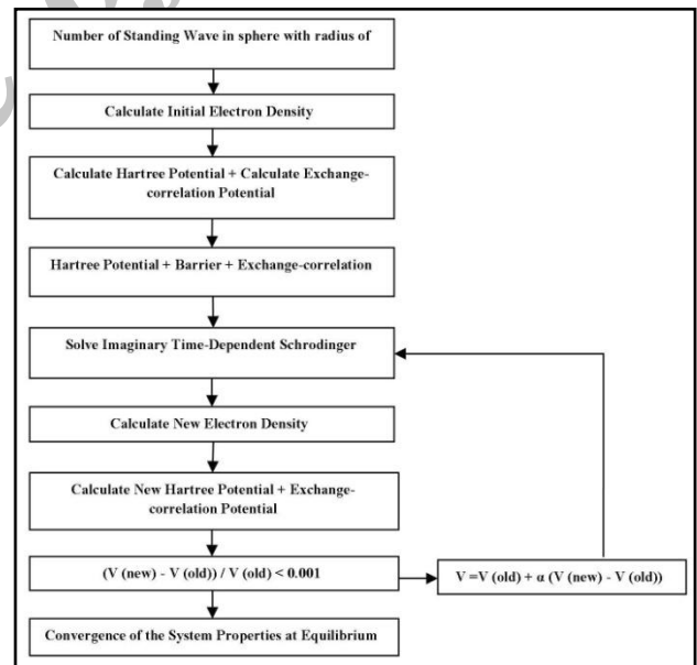
Fig. 2. The flow chart of the process of the closed system at equilibrium
