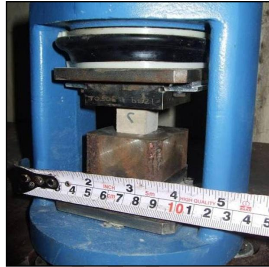
Fig. 4. Testing of the 20-mm paste cubes
