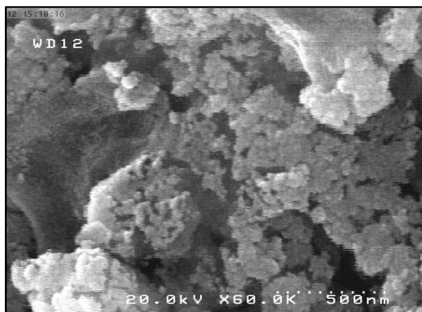
Fig. 3. SEM images of the \text{CoBr}_2 \cdot 6\text{H}_2\text{O} nanoparticles
