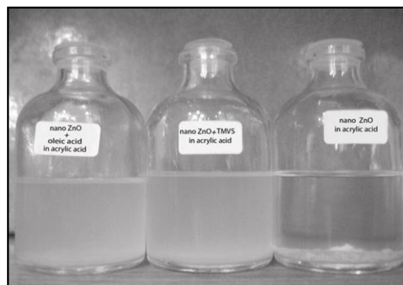
Fig. 3. ZnO nano-particles dispersed in acrylic acid after 24 h under aerobic conditions. Modified with oleic acid (a), with TMVS (b) and unmodified ZnO nanoparticles (c).
