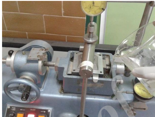
Fig. 13. Performing direct shear test in specimen with saturated condition.
