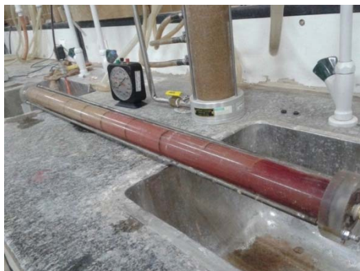
Fig. 7. Injection pipe with L=1m and D=4cm in this study.
