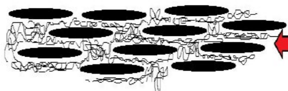
Fig. 4. Slippage of needle like CNC on each other and facilitation of melt flow of LDPE.
