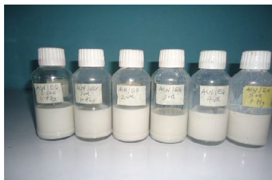
Fig. 2. Photographic image of just prepared AlN/EG nanofluids (0.5, 1, 2, 3, 4 and 5% vol. conc. from left to right).
