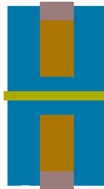
Fig. 4. Top view of proposed FinFET.
