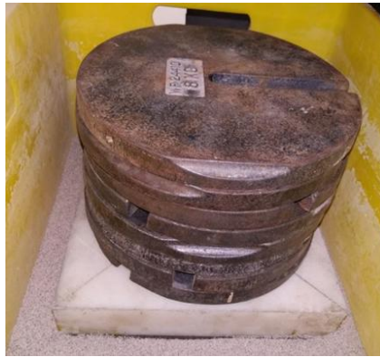
Figure 5. Method of roughening geotextiles
