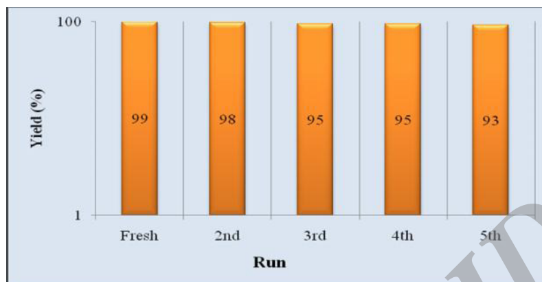
Figure 1. Yield refers to isolated products from the aminopyridines (1 mmol), 4-chlorobenzaldehyde (1 mmol), cyclohexylisocyanide (1 mmol) in the presence of 0.05 g silzic under solvent-free condition.
