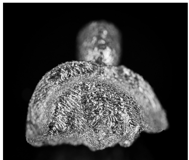
Figure 6. Intaglio view of the additive-manufactured onlay.
