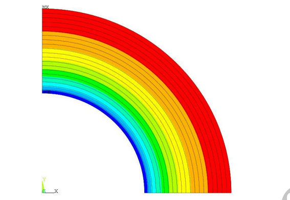
Fig. 8. Radial stress obtained from ANSYS code in an FGM spherical pressure vessel ($\beta = 1$)
