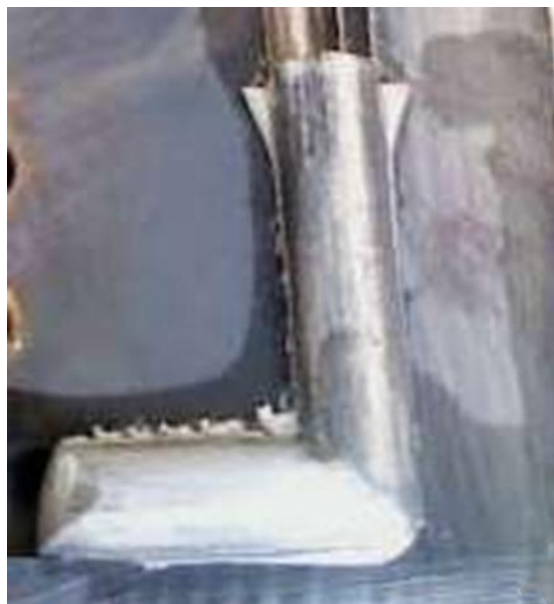
Fig. 9. ECAPed aluminum billet during the process
