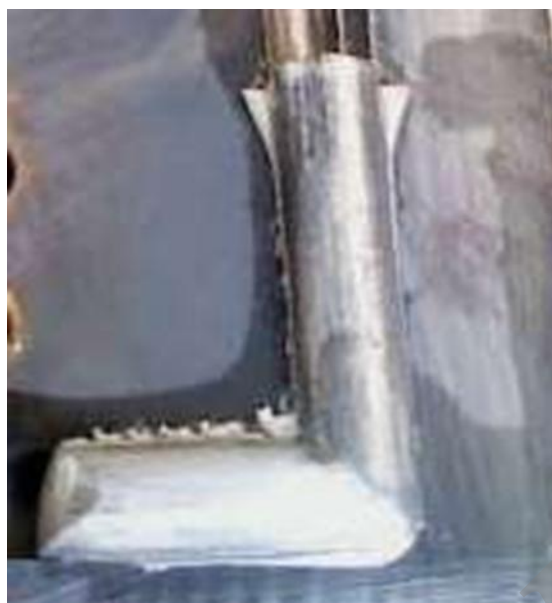
Fig. 9. ECAPed aluminum billet during the process
