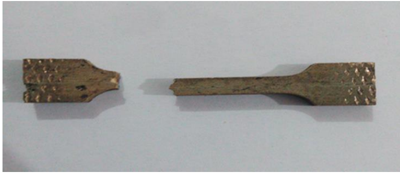
Fig. 11. One of the samples after the tensile test
