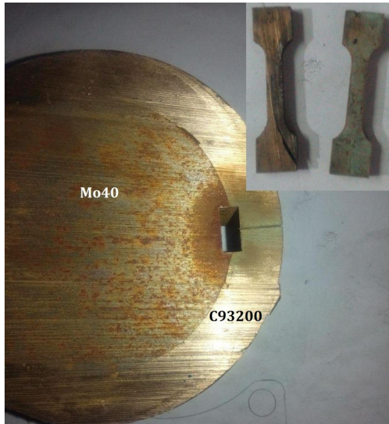
Fig. 3. (a) Tensile test sample map [23] (b) wire-cutted specimen for tensile test
